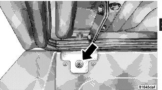
Left Hinge And Attach Bolt
